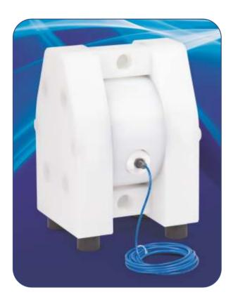
Although DELLMECO diaphragms with integrated metal core are designed for an optimum service life, the diaphragm remains a wear part. If it breaks, liquid can leak into the center housing and possibly emerge through the muffler. This can be prevented simply and effectively with the DELLMECO diaphragm monitoring.
