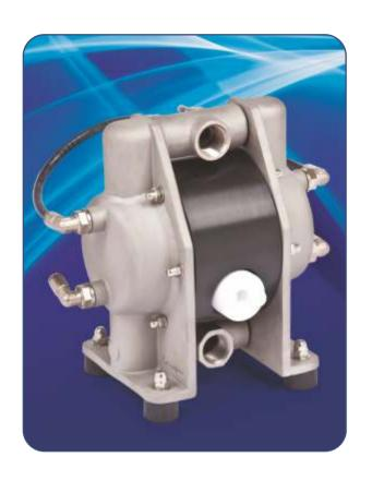
Metal pump with hreating/cooling jacket. The heating/cooling jacket is used when the pumped product has to maintain a specific temperature, high or low, throughout the process. A heating or cooling medium is continuously circulated inside of the jacket. The jacket is covering all the wetted parts of the pump.
