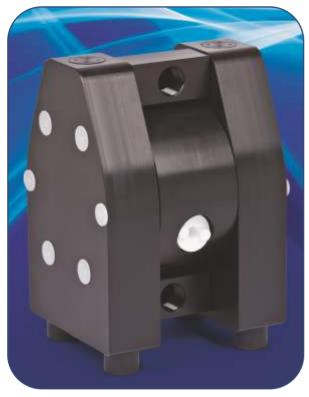
The plastic pumps manufactured of conductive PE and PTFE are constructed to enable grounding of non-metallic pumps. This feature allows the pump to safely transfer solvents, alcohols and other volatile liquids without the danger of static electricity build-up. These features apply also to the aluminium, cast iron and AISI 316 pumps.
