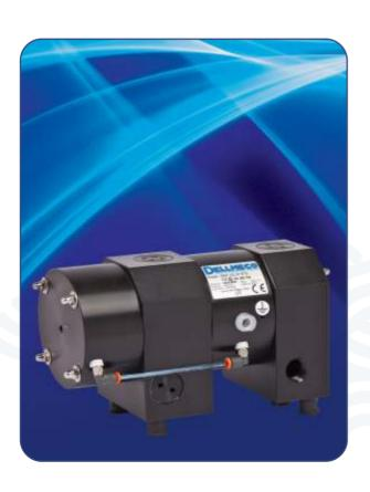
DMF pumps are pneumatic diaphragm pumps with integrated pulsation damper and two separated product chambers. Transport of liquid is realized by the delivery chamber. The fluid passes an active pulsation damper to smoothen the flow. Trouble-free operation of the pulsation damper is only possible with a minimum back pressure of 1 bar and becomes increasingly efficient as the back pressure increases.
