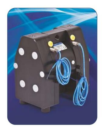
To comply with high safety standards, the barrier chamber system replaces the standard diaphragm by a tandem arrangement of two diaphragms and a barrier chamber of conductive PE filled with a non-conductive liquid in between.
